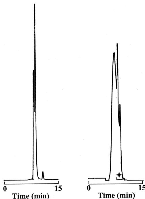
Fig. 2. GPC analysis of (a) phenol standard containing 30  $\mu\text{g}/\text{g}$  eugenol, phenol, catechol, *o*-cresol and creosol in THF (scale 10 mV), and (b) 0.53% (w/w) pyrolysis oil in THF (scale 100 mV). The fraction containing phenols (8–10 min) is marked. The detection wavelength was 270 nm.
