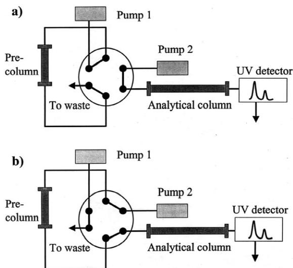
Fig. 1. Steps in column switching (LC–LC). Valve positions during (a) clean-up and pre-fractionation in the pre-column (0–0.5 min) and separation in the analytical column (6 min $\rightarrow$ ), and (b) transfer of the phenolic fraction to the analytical column (0.5–6 min).
